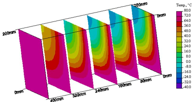
Figure 4: 3D graphics for the temperature distribution in 1/8 of the volume of the subjected to defrosting beech prisms with  $t_0 = -40\text{ }^\circ\text{C}$ ,  $u = 0,3\text{ kg.kg}^{-1}$  (above) and  $u = 0,6\text{ kg.kg}^{-1}$  (below) after 10 h thermal treatment at  $t_m = 80\text{ }^\circ\text{C}$
