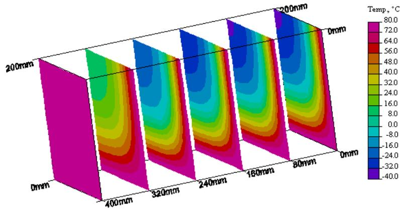
Figure 3: 3D graphics for the temperature distribution in 1/8 of the volume of the subjected to defrosting beech prisms with  $t_0 = -40\text{ }^\circ\text{C}$ ,  $u = 0,3\text{ kg.kg}^{-1}$  (above) and  $u = 0,6\text{ kg.kg}^{-1}$  (below) after 5 h thermal treatment at  $t_m = 80\text{ }^\circ\text{C}$
