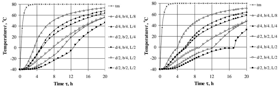
Figure 2: 3D defrosting at  $t_m = 80\text{ }^\circ\text{C}$  of beech prisms with dimensions 0,4 x 0,4 x 0,8 m,  $t_0 = -40\text{ }^\circ\text{C}$ ,  $\rho_b = 560\text{ kg.kg}^{-1}$ ,  $u_{fsp}^{20} = 0,31\text{ kg.kg}^{-1}$ ,  $u = 0,3\text{ kg.kg}^{-1}$  (left), and  $u = 0,6\text{ kg.kg}^{-1}$  (right) depending on  $\tau$
