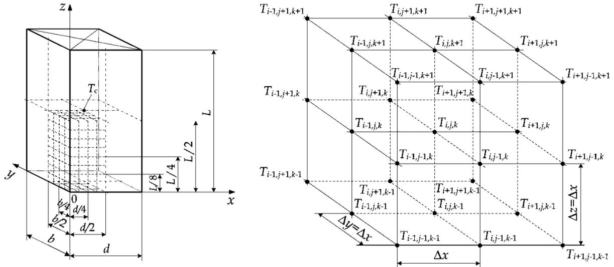
Figure 1: Positioning of the knots in the calculation mesh on 1/8 of the volume of a subjected to thermal treatment frozen wooden prism
