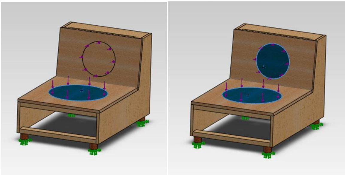
**Figure 4: Scheme of the loads of the supporting structure in an armchair for relax**
