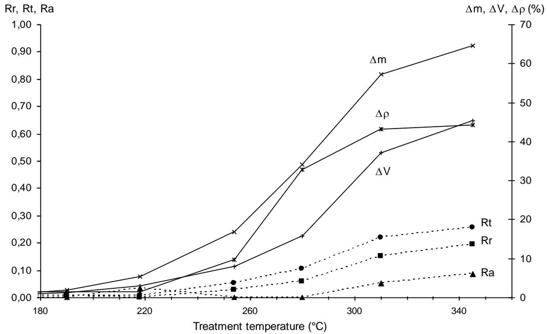
**Figure 6: Evolution of mass, volume, specific gravity and shrinkage as a function of temperature treatment for pine wood**
