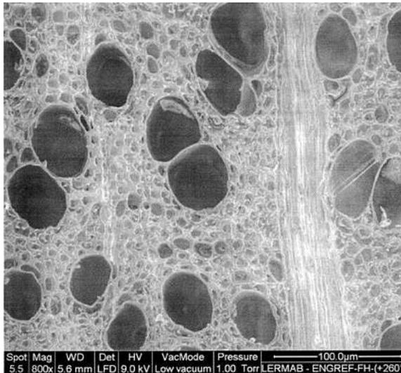
**Figure 2: Transversal plan observation for beech wood after heat treatment (260 °C, 8h)**
