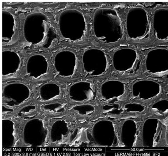
**Figure 4: Transversal plan observation for pine wood after heat treatment (260 °C, 8h)**
