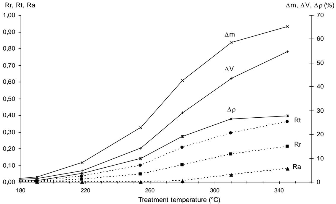
**Figure 5: Evolution of mass, volume, specific gravity and shrinkage as a function of temperature treatment for beech wood**
