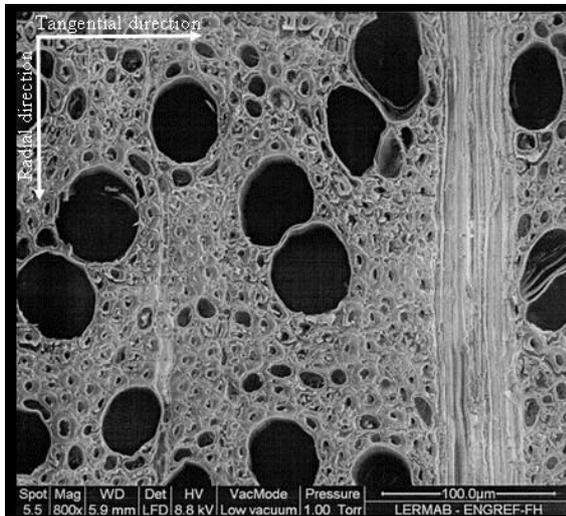
**Figure 1: Transversal plan observation for beech wood**
