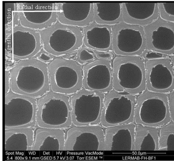
**Figure 3: Transversal plan observation for pine wood**
