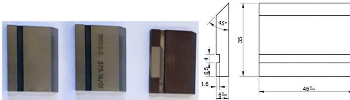
Figure 1: Changeable milling knives and their dimensions
