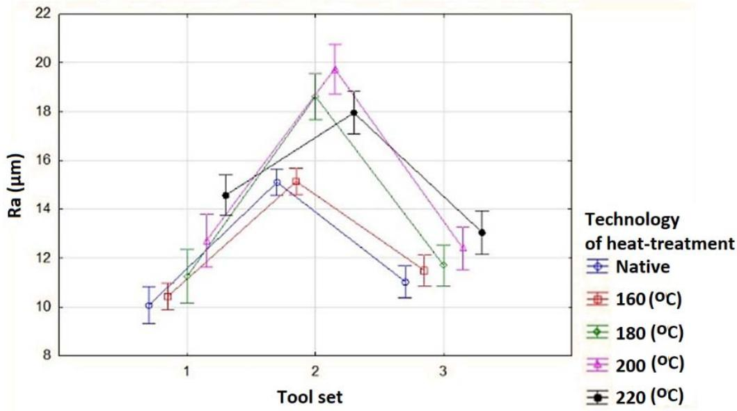
Figure 4: Effect of heat-treatment technology and tool set on surface roughness
