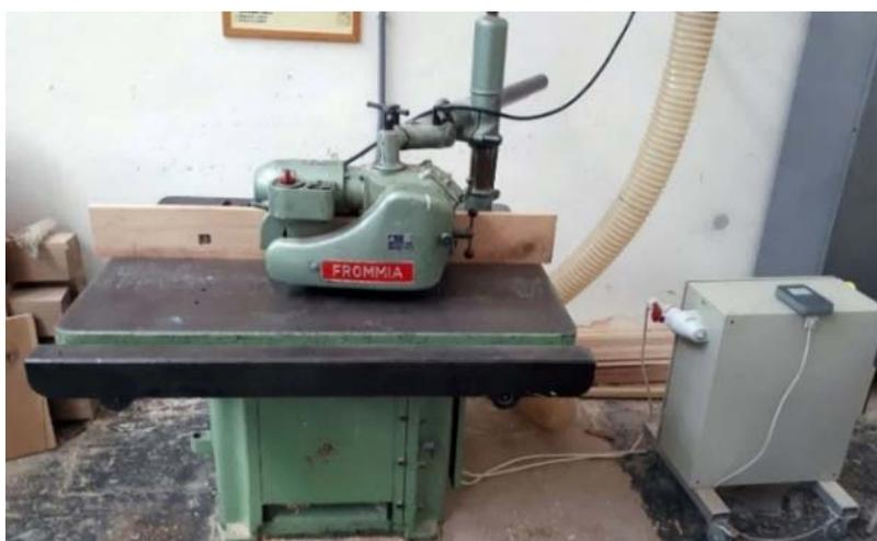
Figure 2: Lower milling machine FVS with feeder Frommia ZMD 252/137
