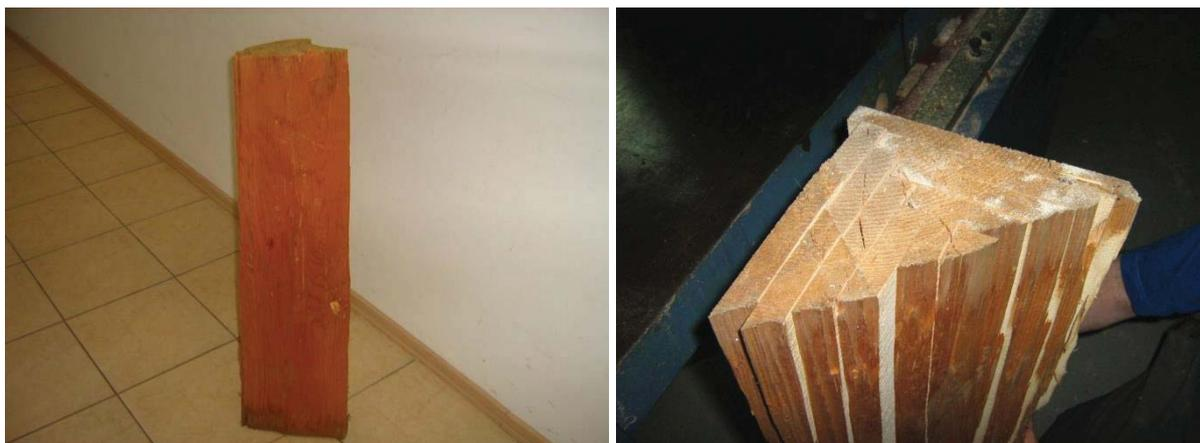
Figure 1: General view of the blank (left) and a cutting scheme (right).
