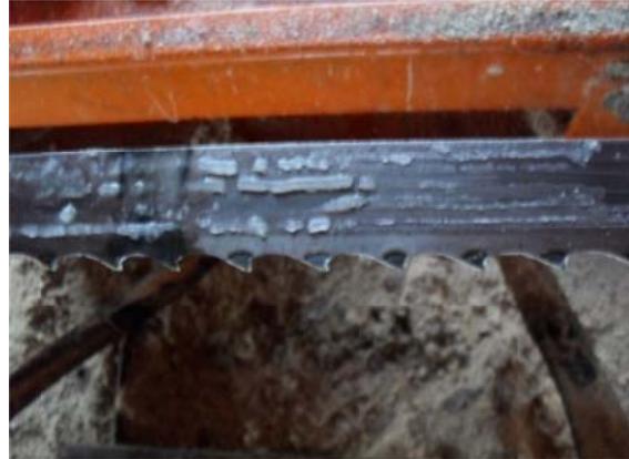
Figure 10: Freezing of the cleaning liquid on a saw blade
