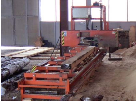
Figure 1: General view of a horizontal band saw “Wirex”, model “CZ-1/ZM” (Poland)
