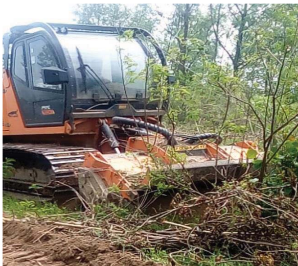
Figure 1: PT 400 specialized milling unit with FAE300S multi-purpose forestry tiller (Photo K. Marinov)
