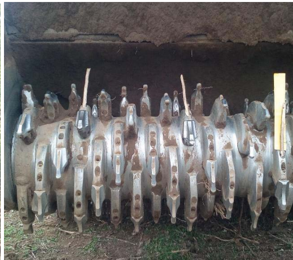
Figure 1: PT 400 specialized milling unit with FAE300S multi-purpose forestry tiller (Photo K. Marinov)
