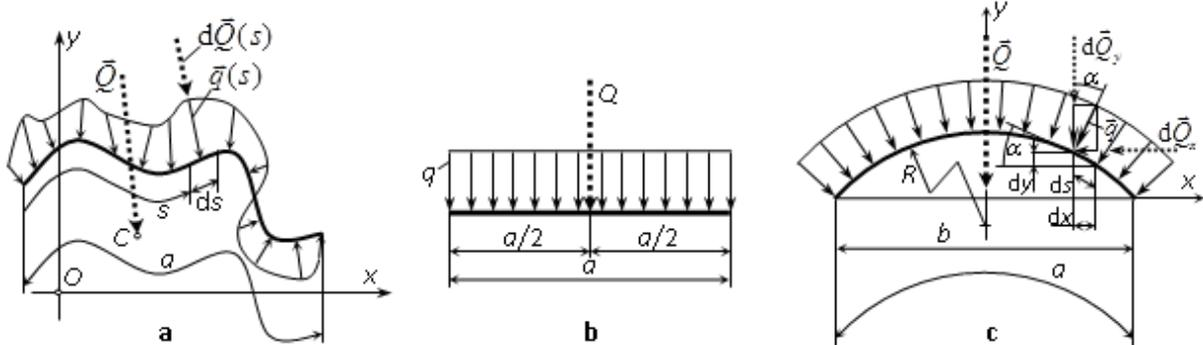
Figure 3: Illustrations to the concentration of distributed forces
