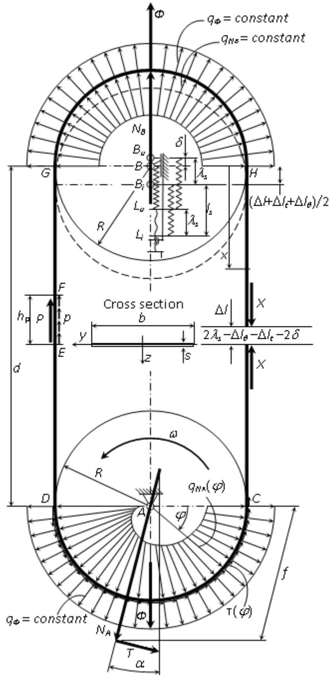
Figure 1: Scheme for determination of  $X$  of a vertical bandsaw
