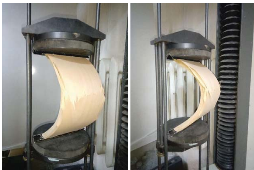
Figure 4: Test samples lined with 0.6 mm beech veneer.
