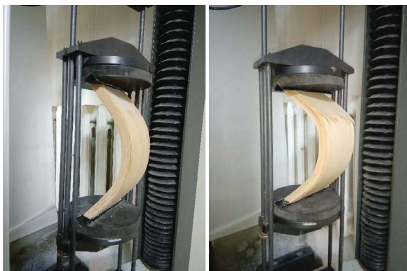
Figure 5: Test samples lined with 2 mm oak veneer.
