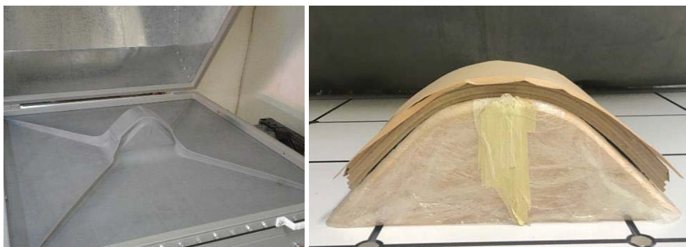
Figure 1: Laboratory vacuum press and the matrix for bending with a radius of curvature of 100 mm
