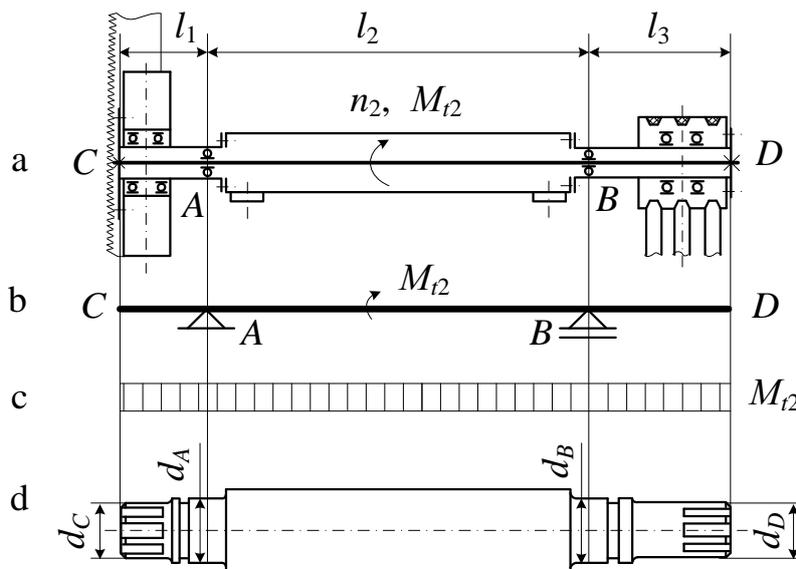
Figure 6: Calculation scheme and diagrams of the torque and the construction of the main band saw shaft
