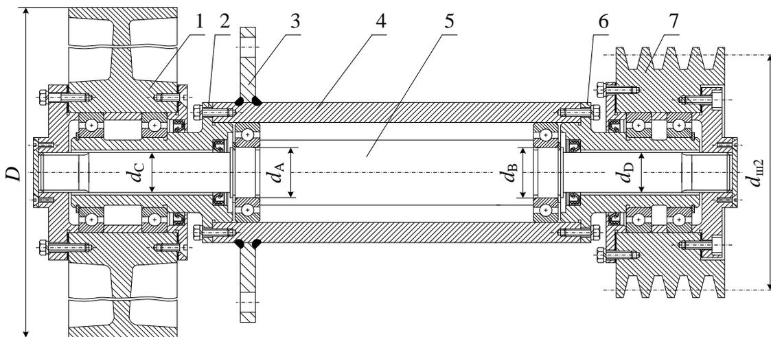
Figure 7: Construction of the main band saw shaft submitted to torsion
