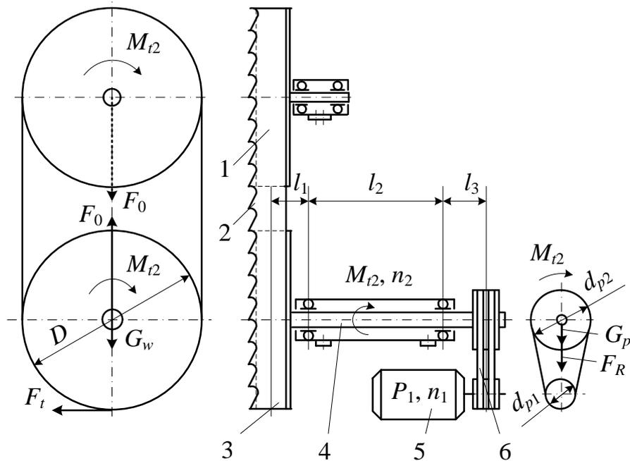
Figure 1: Cutting mechanism of band-saw machine
