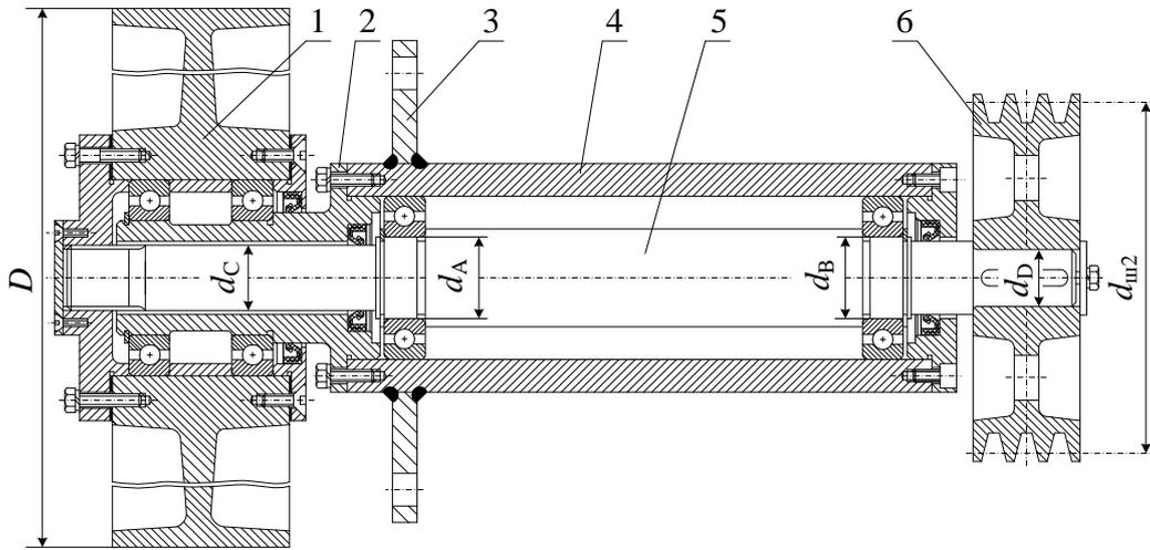
Figure 5: Construction of the main band saw shaft submitted to bending by the tension force of the belts and to twisting
