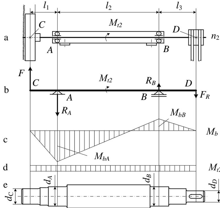
**Figure 2: Calculation scheme and diagrams of bending and twisting moments and construction of the main band saw shaft.**
