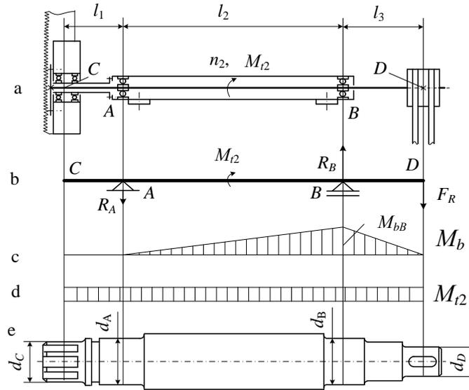
**Figure 4: Calculation scheme and diagrams of the bending moment and torque and the construction of the main band saw shaft**
