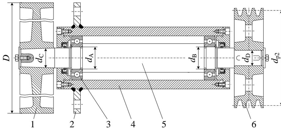
Figure 3: Design of the main band saw shaft submitted to bending by the tension forces of the band and the belts and submitted also to twisting
