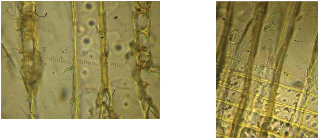
**Figure 3: Core rays and mechanical cells in a tangential section (left) and a radial section (right) of a thermally modified wood of spruce, x400.**
