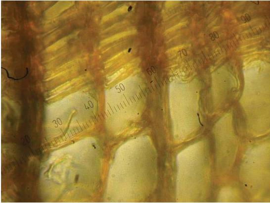
wood. The fragmentations of the cell wall have probably been obtained during the preparation of the sample.
