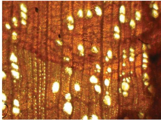
**Figure 8: Cross section (with optical zoomx32) of natural hornbeam wood (left) and thermally modified (right).**
