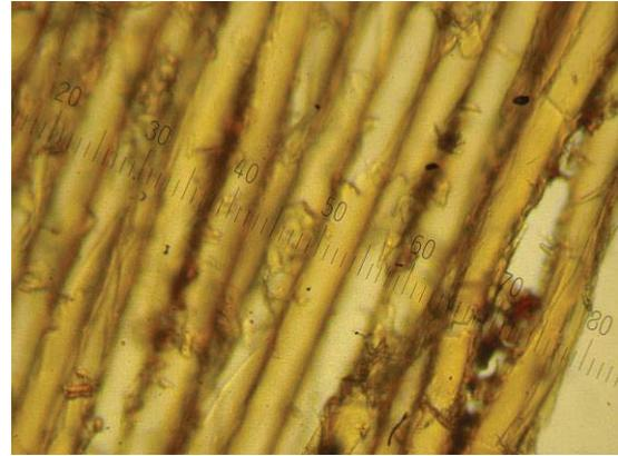
**Figure 4: Cross (left, x400) and tangential (right, x100) section of thermally modified pine wood.**
