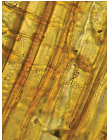
Figure 7: Core rays and mechanical cells in tangential section(left)and vessels, fibers and rays in radial section (right) of thermally modified oak wood with optical zoomx400.
