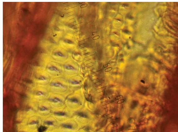
Figure 11: Core rays and mechanical cells in tangential section (left) and vessels in radial section (right) of thermally modified birch wood with optical zoom x400.
