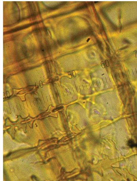
**Figure 5: Core rays and tracheids in radial section of thermally modified pine wood with optical zoom x100 (left) and x400 (right).**
