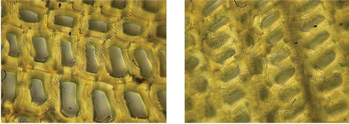
**Figure 2: Cross section (x400) of natural (left) and thermally modified wood of spruce (right).**
