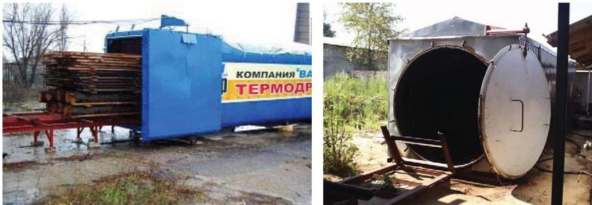
Figure 1: The thermoconvective – SPCT (left) and vacuum – SPVT (right) heat treatment dryer.
