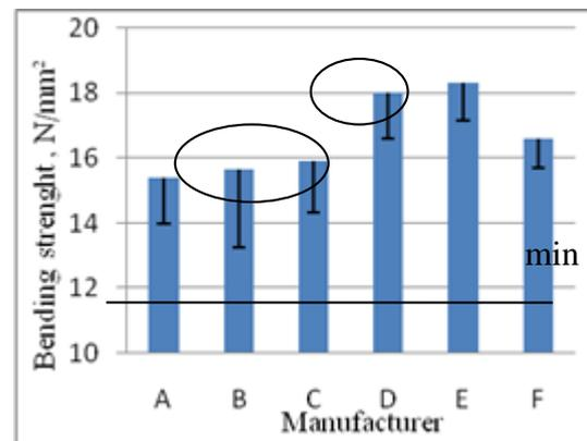
**Figure 1: Bending strength and lower limit of the confidence interval**
