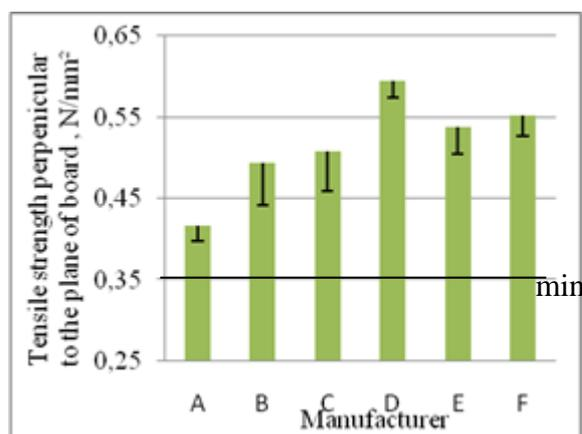
**Figure 2: Tensile strength perpendicular to the plane of the board and lower limit of the confidence interval**
