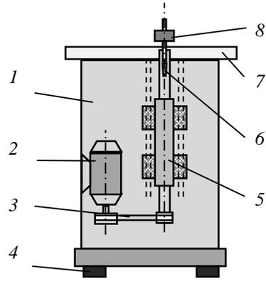
Figure 1: Wood shaper – general view Figure 2: Scheme of wood shaper
