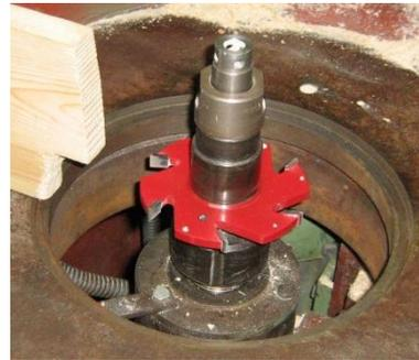
Figure 3: Spindle with bearing units and with cutter
