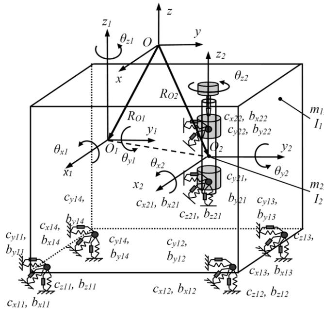
**Figure 5: Mechanic-mathematical model for investigation of the free damped spatial vibrations of the woodworking shaper and its spindle**
