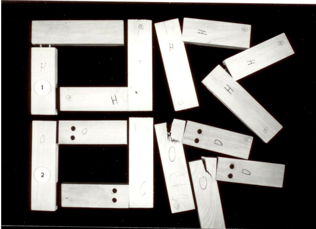
Figure 5: Typical way of destruction of dismountable end corner joints of components made from solid beech wood under bending load: 1 – with two one-piece connectors “Confirmat”; 2 – with two connectors with screw and cross dowel.
