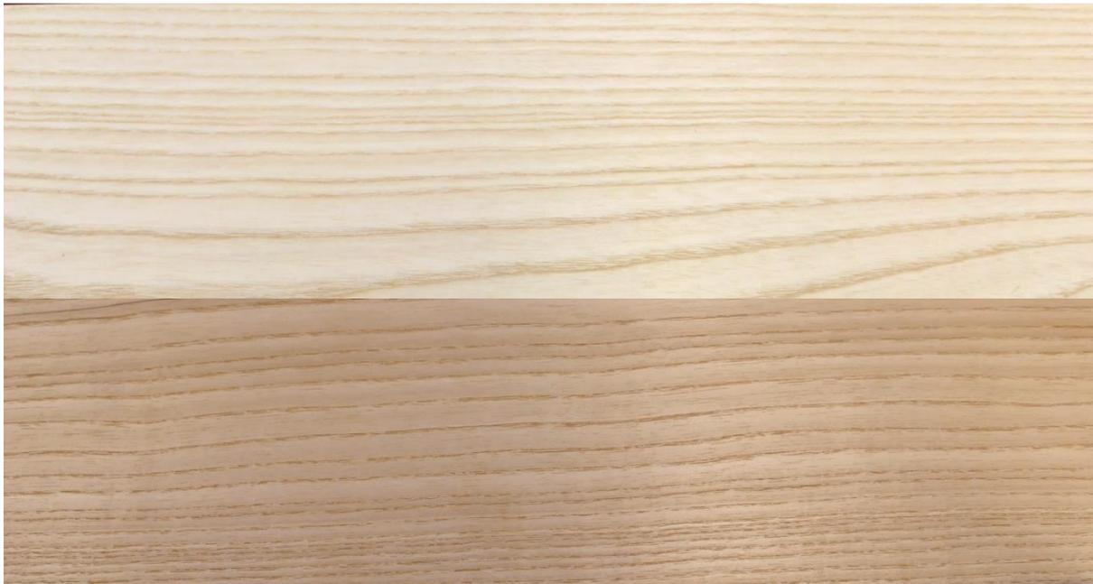
**Figure 2: View of the European ash wood before and after thermal treatment**
