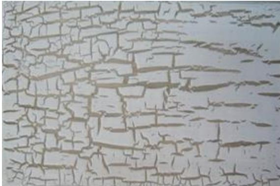
Figure 8: Effect „crackle“ on ash
