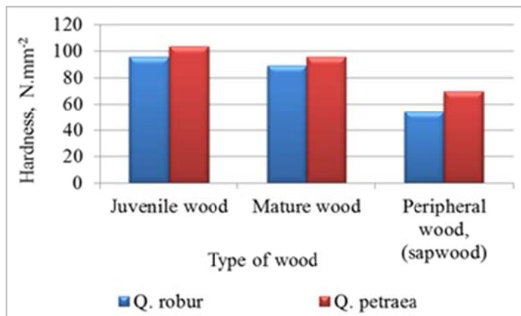
Figure 3: Distribution of hardness depending the radius of the stem
