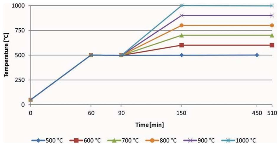
Figure 2: The temperature profile of the sample heating and combustion of biofuels in a muffle furnace
