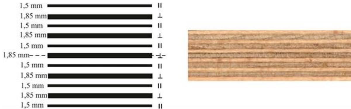
Figure 1: Pattern and cross-section of plywood structure
