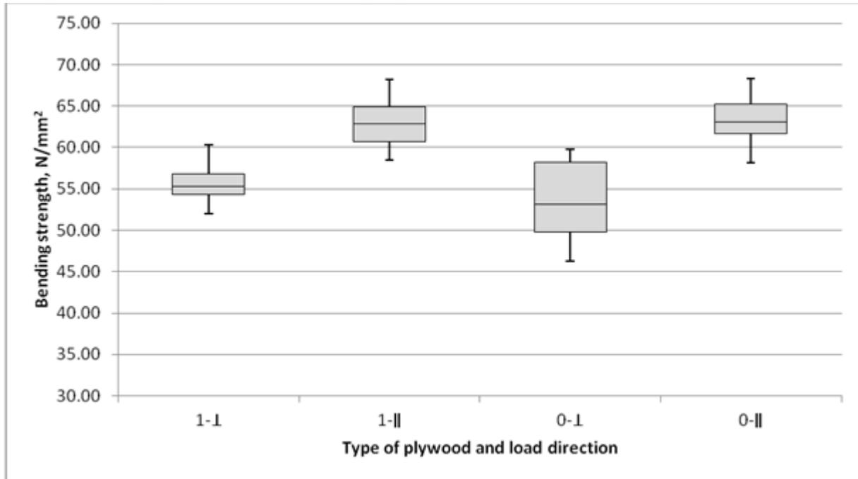
**Figure 3: Bending strength of two types of plywood under loadings perpendicular and parallel to the layers**
