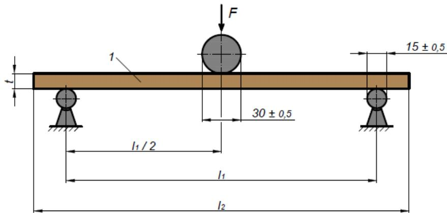
Figure 1: Testing method of panels to determine the modulus of elasticity in bending and bending strength perpendicular to the panel surface: 1 – test sample; F – load; t – thickness of the test sample;  $l_1 = 20t$  mm and  $l_2 = l_1 + 50$ . Dimensions are in mm.
