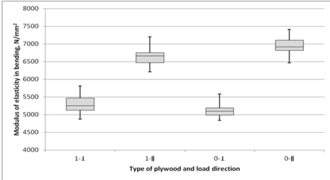
Figure 2: Modulus of elasticity in bending of two types of plywood under loadings perpendicular and parallel to the layers
