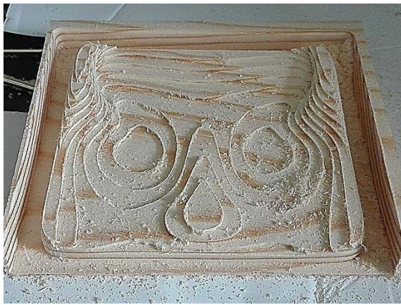
Figure 3: Physical model after roughing operation
