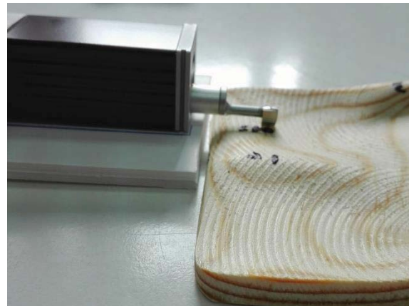
Figure 6: Physical model during the roughness test
