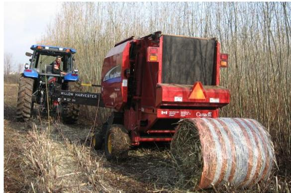
Figure 4: New Holland prototype cutbaling machine
