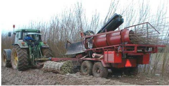
Figure 3: Bundler's prototype – Nicholson cut and bundle harvester
