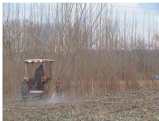
**Figure 2: Cut-only (simple) harvester. SAF – ISMA prototype on two years old poplar**
