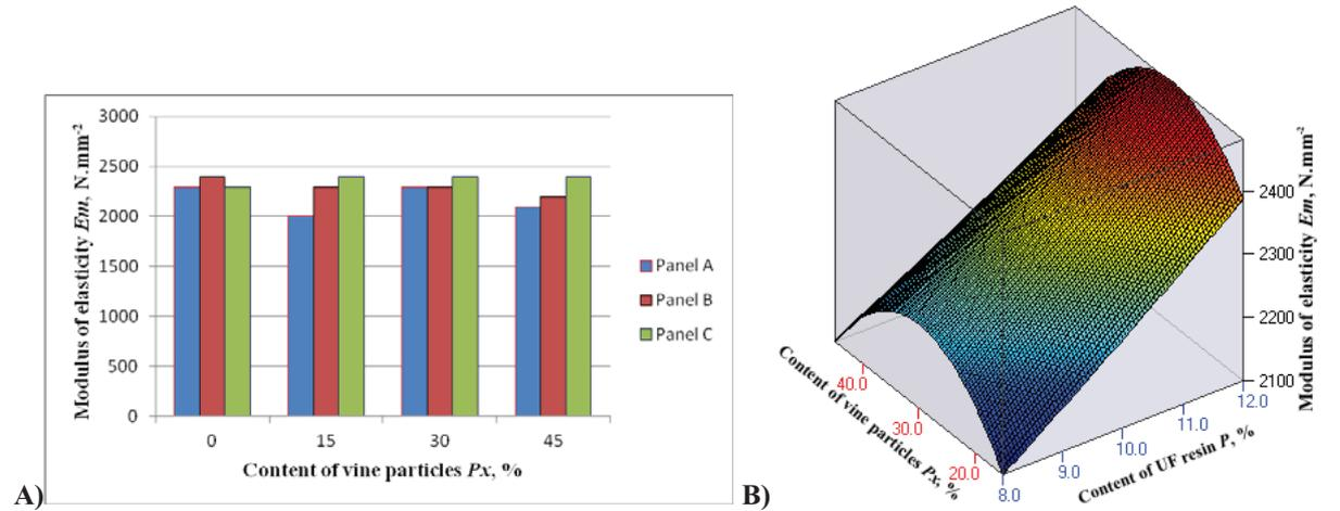
Figure 5: Modulus of elasticity of combined wood-based panels
