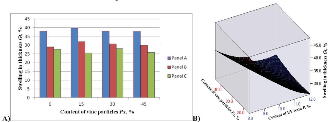
**Figure 3: Swelling in thickness of combined wood-based panels**
