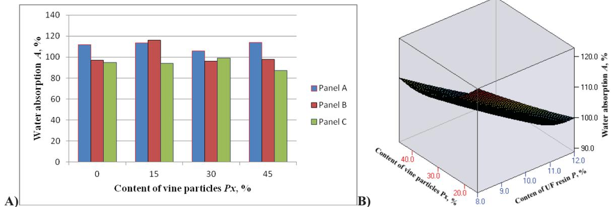
Figure 2: Water absorption of combined wood-based panels
