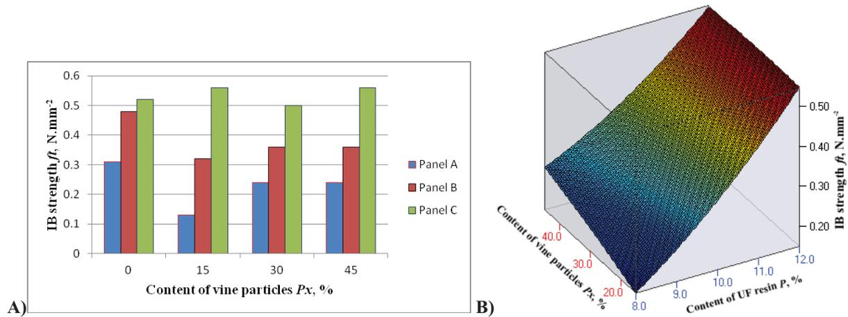
**Figure 6: Internal bond strength of combined wood-based panels**
