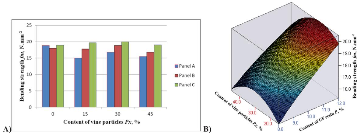
**Figure 4: Bending strength of combined wood-based panels**
