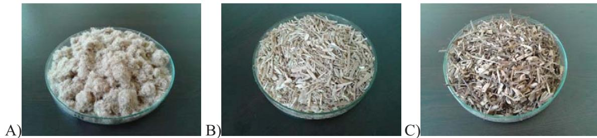
**Figure 1: Materials used for the production of combined wood-based panels A) wood fibres; B) wood particles; C) vine particles**
