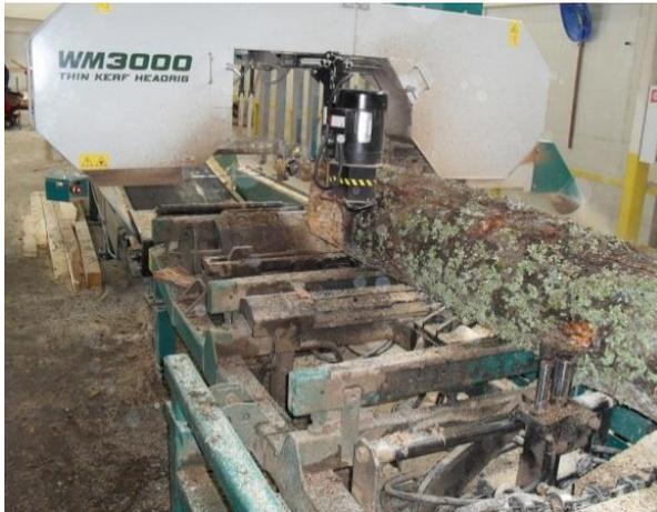
Figure 1: Horizontal band saw, model WM 3000
