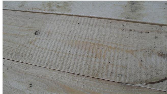
**Figure 6: Surfaces after 100 min operation without changing the cutting tool**
