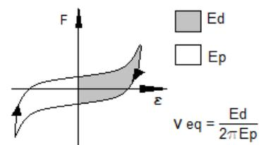
**Figure 2: Typical “load – deformation” curve of mechanical joint in timber structure under cyclic loading. Dissipation of energy in a loading cycle.**
