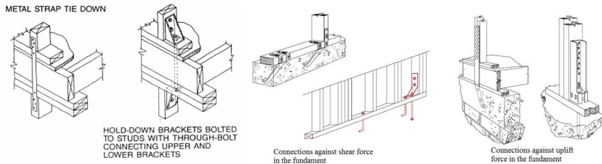
Figure 5: Anchorage connections
