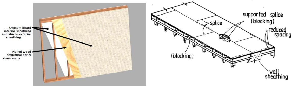
Figure 3: Example of a shear wall and floor construction
