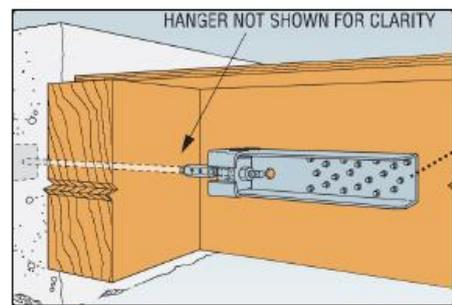
Figure 1: Stress condition "tension perpendicular to the grain" should be avoided
