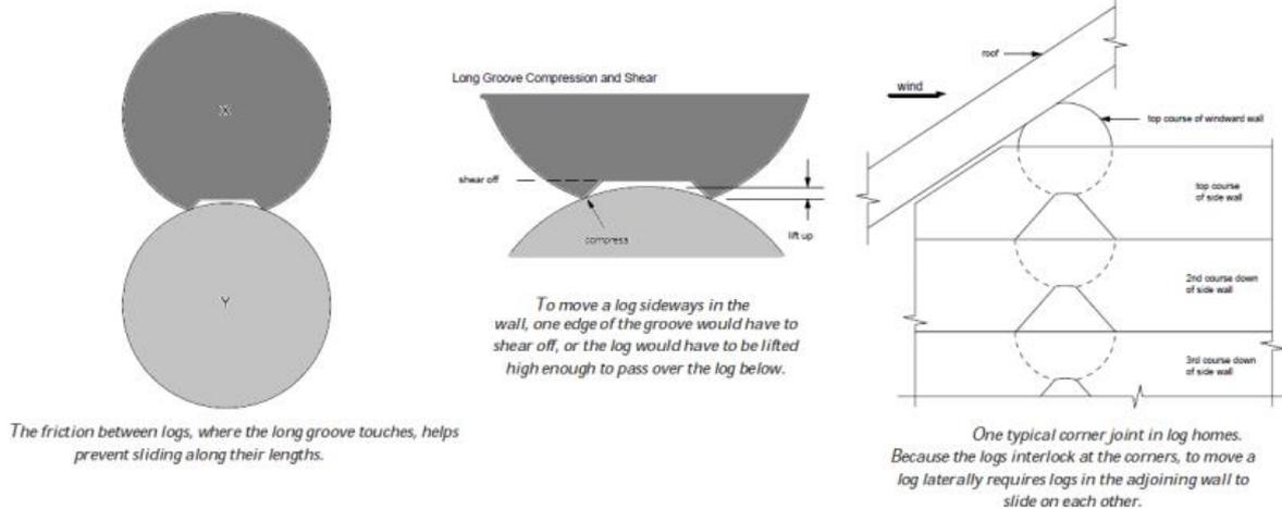
Figure 7: The joineries between logs are providing the lateral stability of the building
