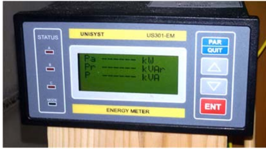
Figure 4: Measurement device US301EM of Unisyst Engineering Ltd. – Bulgaria
