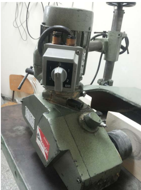
Figure 2: General view of the roller feeder
