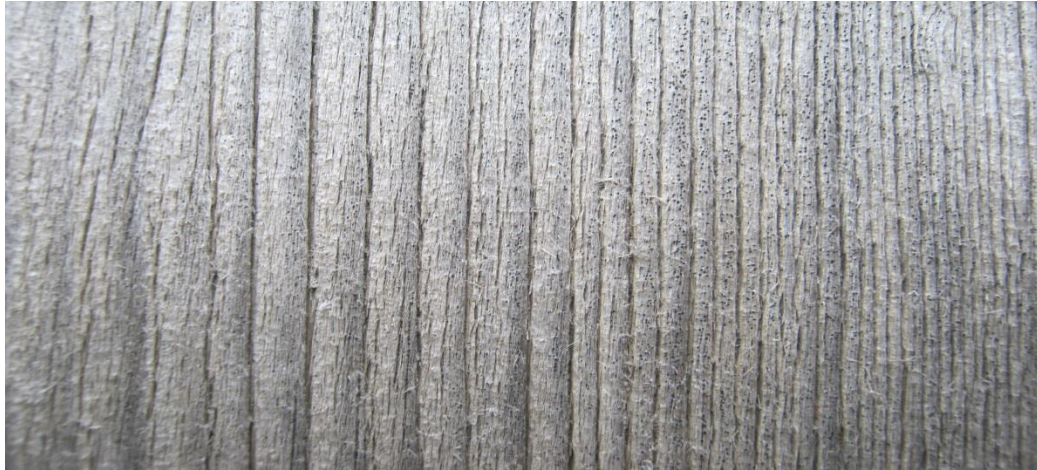
Figure 1: Spruce wood sample 5 years outdoor exposed
