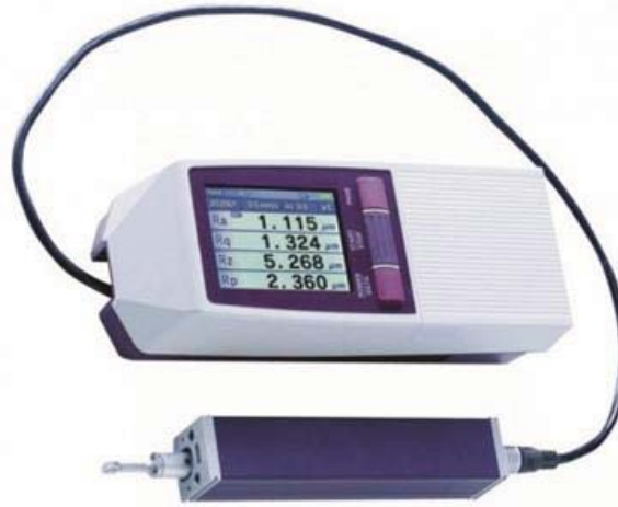
Figure 2. Roughness tester, model SurfTest SJ-210 – general view
