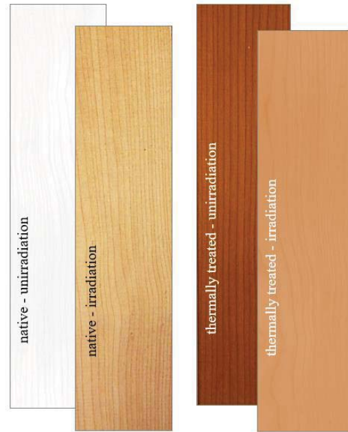
Figure 2: View of maple wood: a) natural before and after UV irradiation, b) thermally treated before and after UV irradiation.
