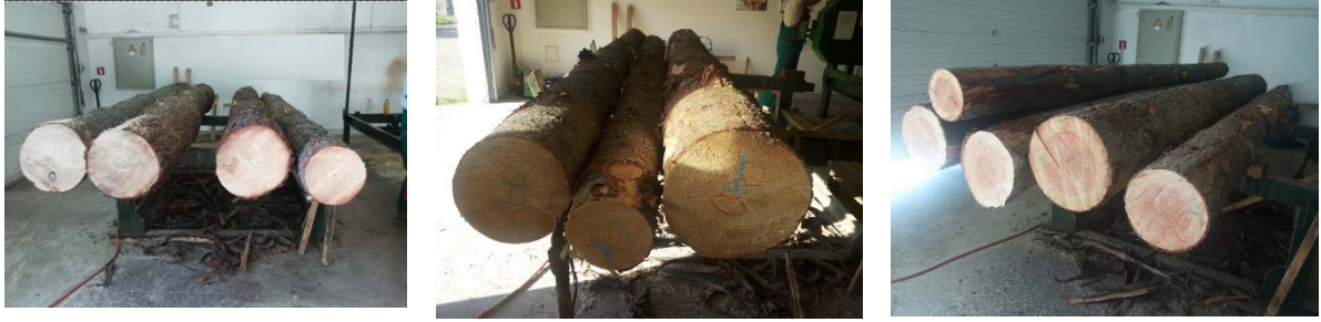
Figure 2: Logs of Scots pine ( Pinus sylvestris L.), Spruce ( Picea abies (L.) Karst.) and Douglas fir ( Pseudotsuga menziesii (Mirb.) Franco)
